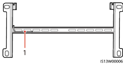
Figure 4-9 Position for binding the security Torx wrench
